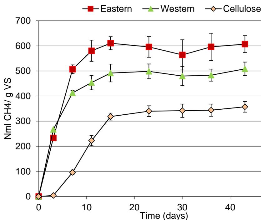
*Figure 15. Average accumulated methane produced per amount of added organic matter (VS)*
