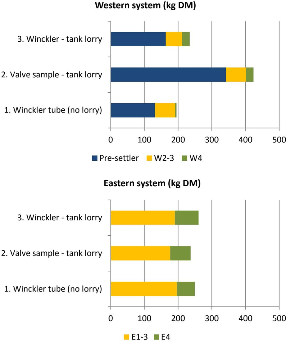
Figure 5. Amount of dry matter that the different parts of each system would contain according to the three different sampling methods.
