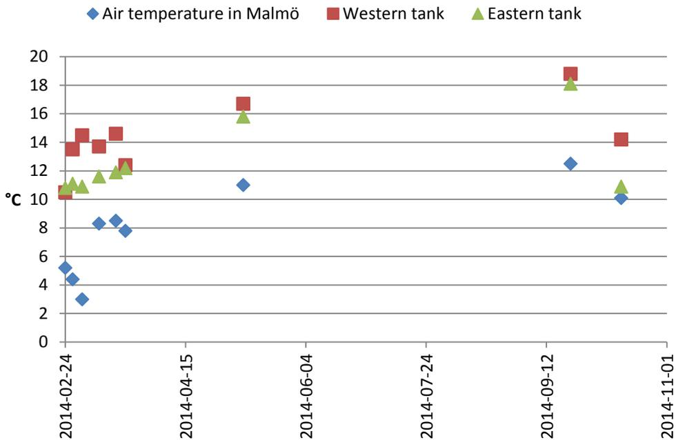
Figure 12. Registered temperatures in the tanks during the sampling periods and corresponding air temperatures.
