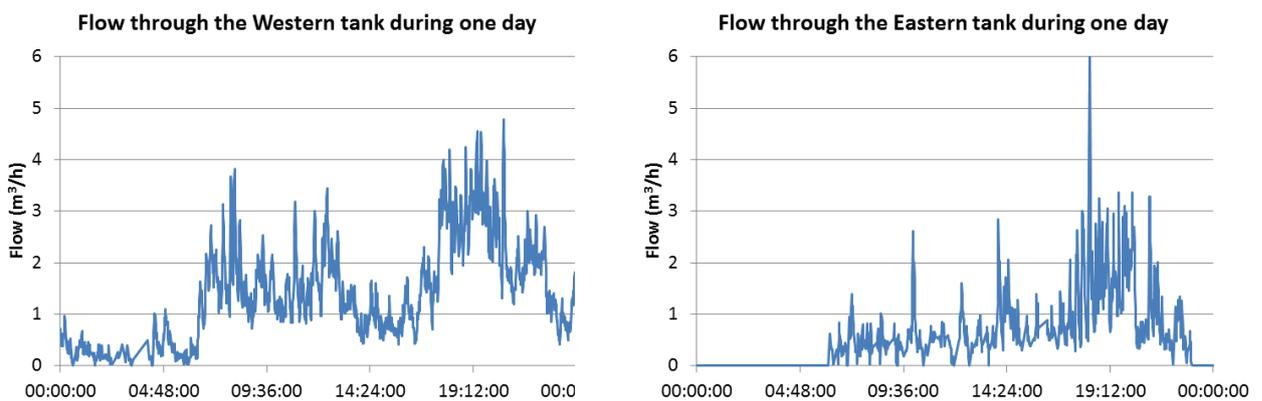
Figure 13. Flow variation during a “typical” 24-hour period (17th of March 2014) for the two tank systems.
