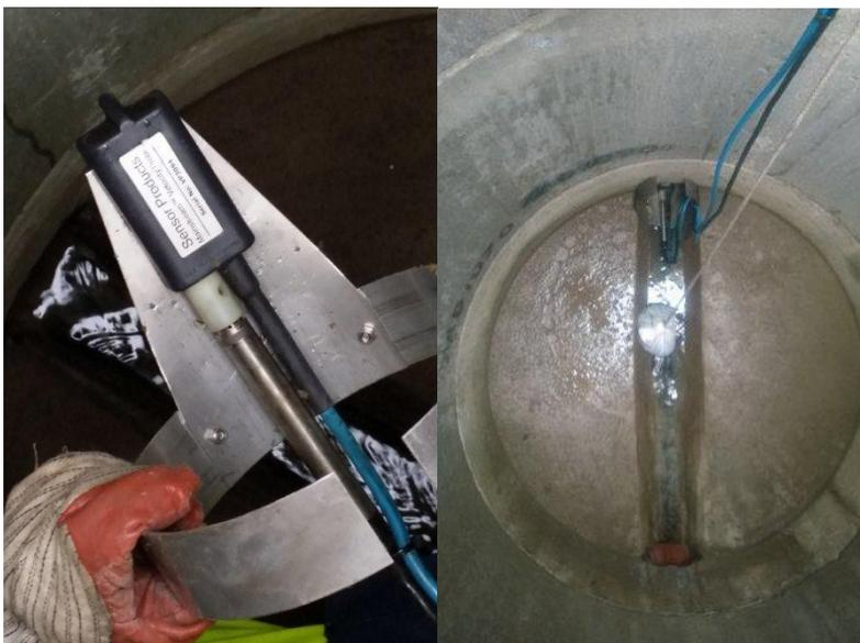
Figure 7. Flow measurement sensor (left) and the installation in the outlet channel (right) with a sand bag for damming up the water level.
