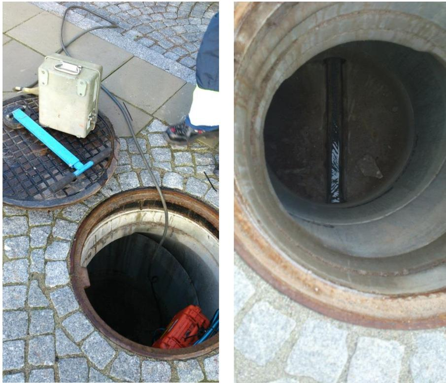
Figure 6. Pump (left) used for sampling from the outlet channel (right)
