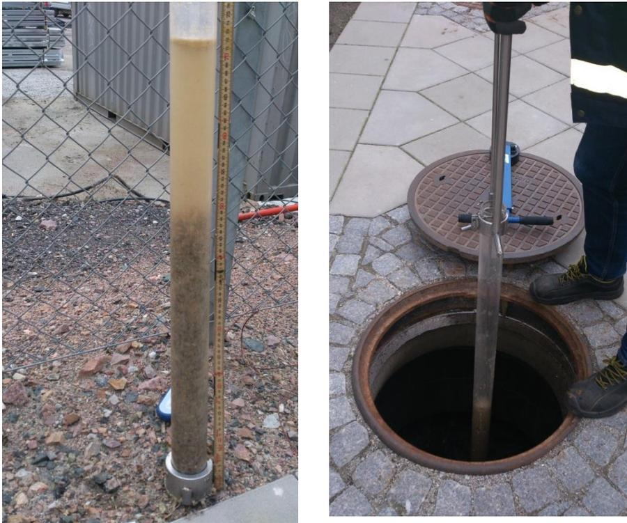
*Figure 4. Sample taken out with the Winckler tube (Method 1)*
