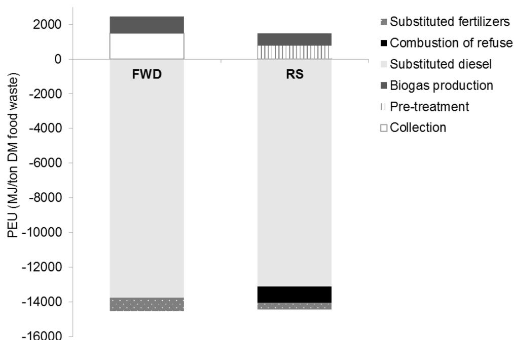
Figure 17. Energy balance (as primary energy use, PEU) in compared systems. FWD = Food waste disposer system. RS = Reference system. The category “Collection” includes material and energy needed for disposal.
