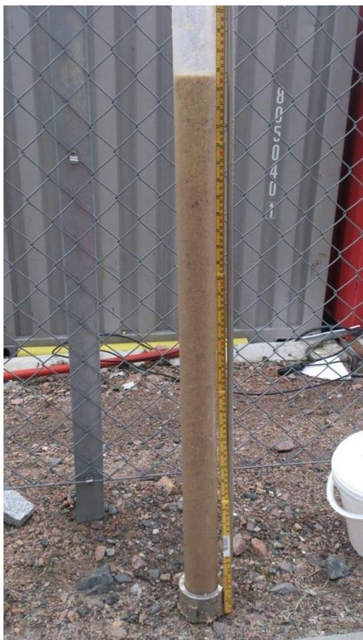
*Figure 11. Sample taken out from the fourth compartment of the Eastern tank after 25 days.*
