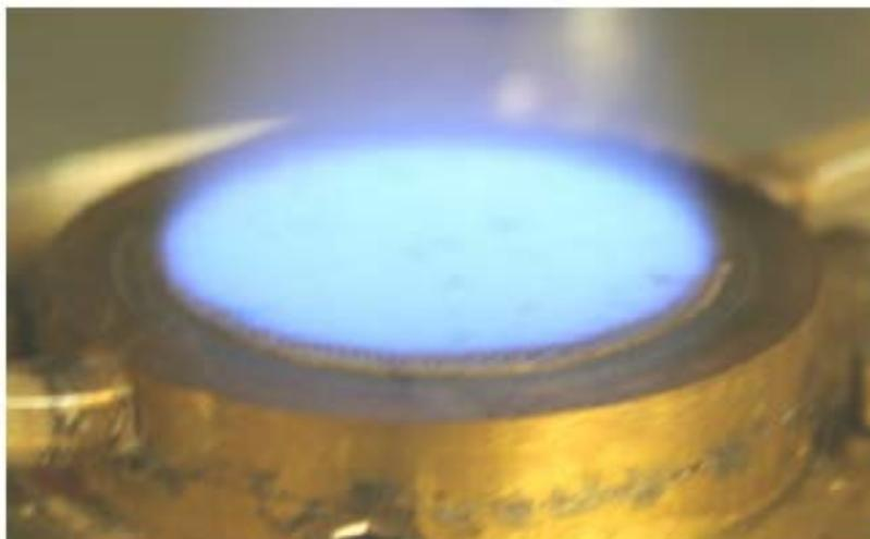
Figure 3. A 1D flame stabilized on a heat flux burner.
