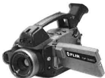
Figure 1. Optical gas imaging camera (FLIR GF 320).
