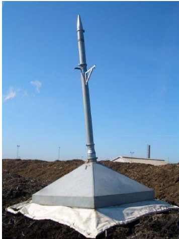
Figure 3. Sampling hood for biofilters.
