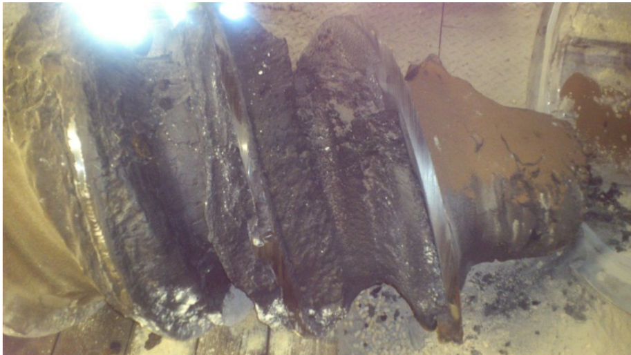
Carbonisation in the feedings screw
