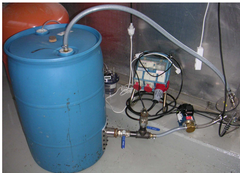
Figure 3: Barrel with pump, gas meter (background) and ultrasonic equipment (right) used in the degassing experiment.
