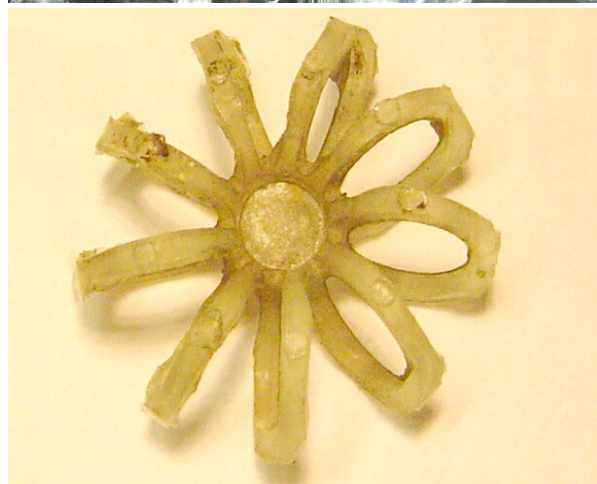
Figure 5. Pall-rings collected from the top left: a) Linköping, most of the culture has been removed from the pall-rings. b) Kristianstad, pall-rings as they looked when collected from the absorption column. c) Uppsala pall-rings have a reddish colour caused by the microbial growth on them. d) Pall-ring that has been used in the Kalmar plant, notice that it is worn. e) A Jönköping pall-ring with the remaining of dark brown microbial growth on it. (Photo: a, d & e: D. Tynell, b: R. Johansson and c: Å. Tynell). Note that the pall-rings are not shown in natural size.
