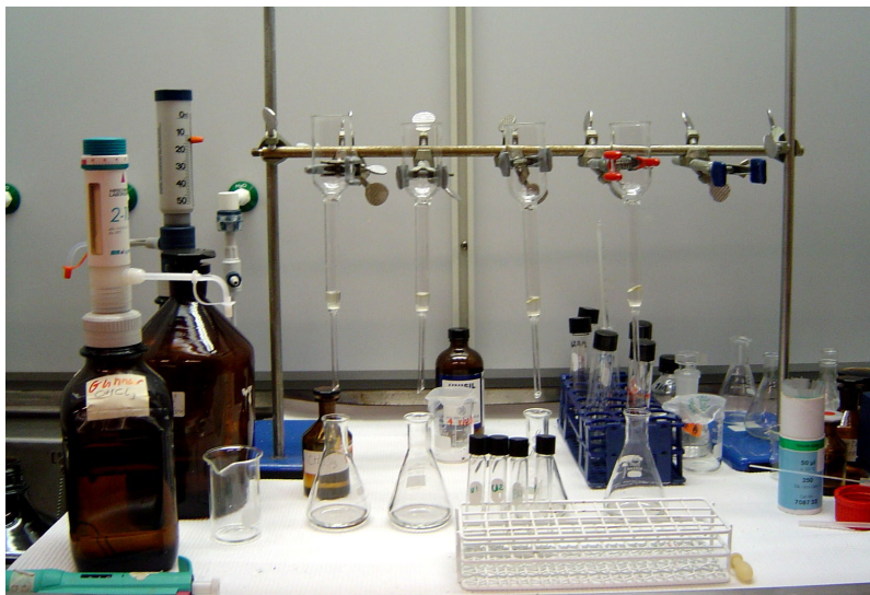
Figure 8. Extraction of the polar lipid phase from the samples. (Photo: Å. Tynell)
