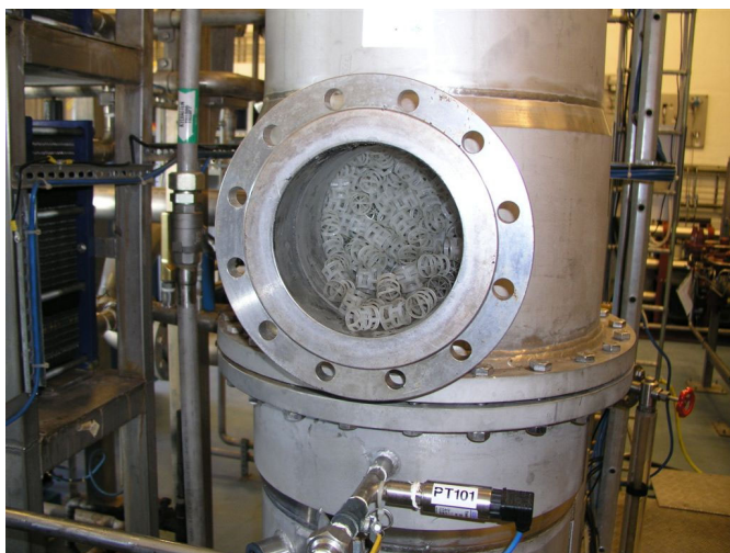
Figure 6. The lower opening of the absorption column of the Kristianstad plant. The column is filled with pall-rings. (Photo: R.. Johansson)
