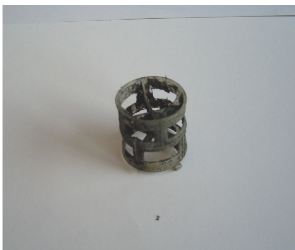
Figure 5. Pall-rings collected from the top left: a) Linköping, most of the culture has been removed from the pall-rings. b) Kristianstad, pall-rings as they looked when collected from the absorption column. c) Uppsala pall-rings have a reddish colour caused by the microbial growth on them. d) Pall-ring that has been used in the Kalmar plant, notice that it is worn. e) A Jönköping pall-ring with the remaining of dark brown microbial growth on it. (Photo: a, d & e: D. Tynell, b: R. Johansson and c: Å. Tynell). Note that the pall-rings are not shown in natural size.
