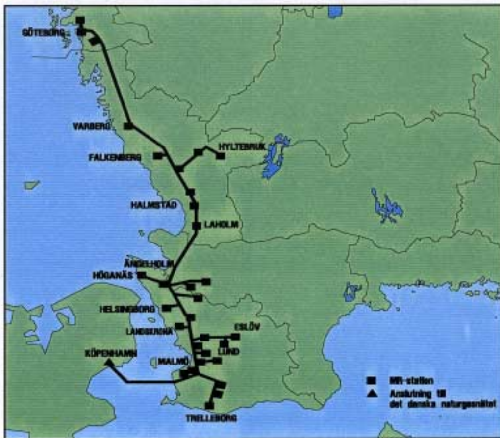
Figure 5 The Swedish high-pressure network for natural gas with MR stations
