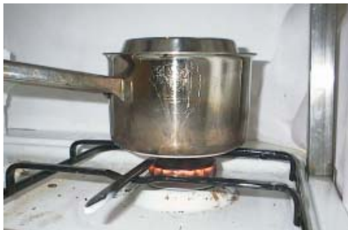
Fig. 4. Example of catalytic combustion gas stove burner.
