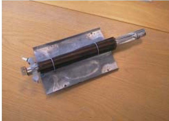
Fig. 3. A folded catalytic wire-mesh (fcwm35) mounted downstreams the flame port plate of the burner placed in the oven. To clarify how the catalyst was attached to the burner/port plates, the photo shows the burner in an up-side down position.
