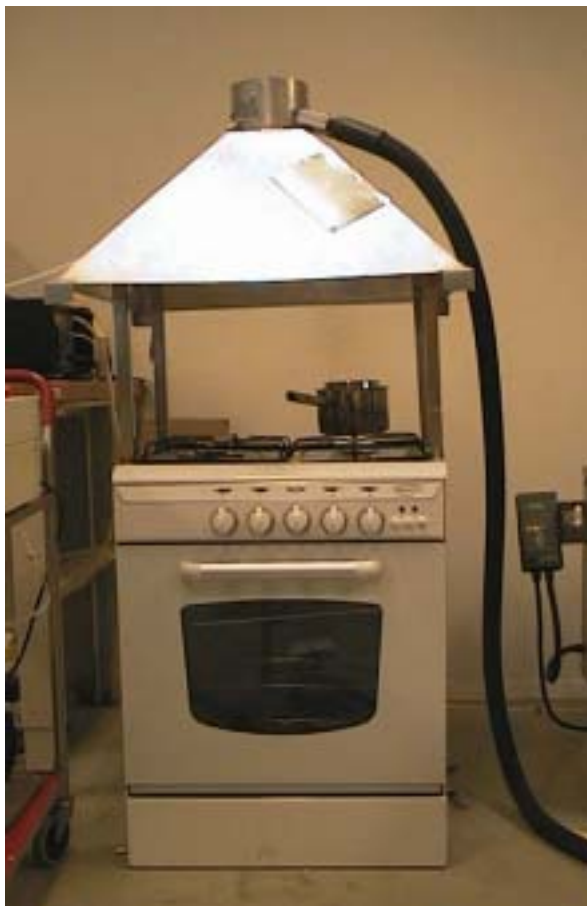
Fig. 2. Gas stove with hood mounted for collecting the emissions in the flue gases.
