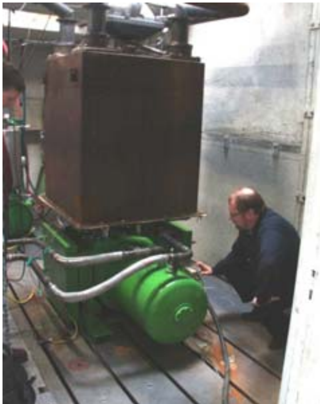
Stirling engine with bio-mass heater on top in the laboratory of the Technical University of Denmark
