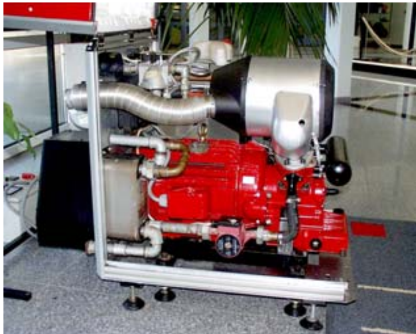
V161 CHP-unit with hood folded back showing; heater unit (grey), Stirling engine (below heater unit), generator, cooling water plate heat exchange and internal cooling water pump.
