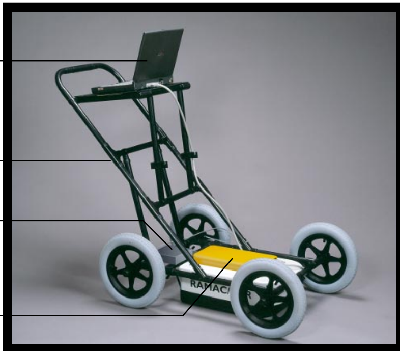
Cart mounted RAMAC X3M with a 500 MHz shielded antenna.
