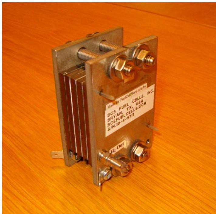
**Figure 6.** A photo of the fuel cell stack used for the PEMFC verification tests performed within this work.
