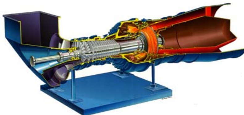
Figur 2. Siemens SGT800 gasturbin [3]
