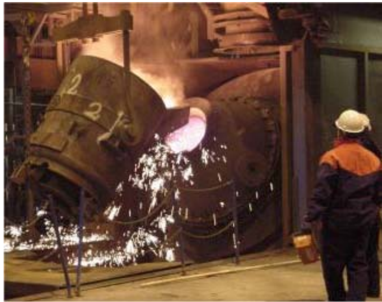
Left, the universal converter at Mefos. Right, charging the tilted converter with the molten metal
