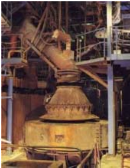
Left, the universal converter at Mefos. Right, charging the tilted converter with the molten metal
