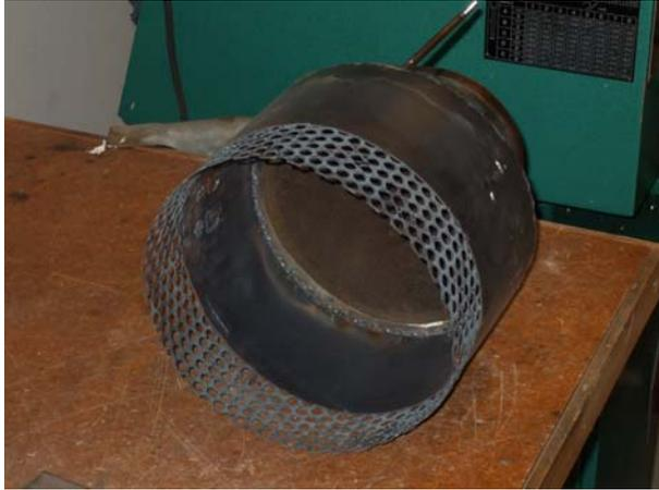
Figure 21 Axial catalytic burner ( $\varnothing$  180 mm)
