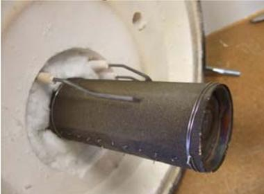
Due to increased surface temperature in catalytic combustion, the original burner head metal became too hot and caused flashback. Thus, data are only recorded at higher loads.
