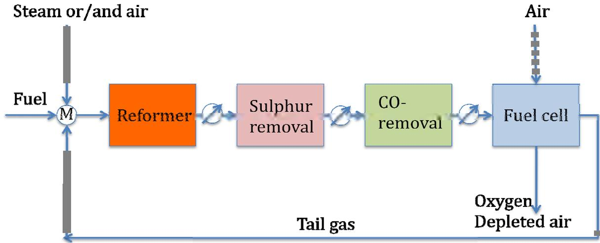
Figure 3 Block diagram, fuel to electricity
