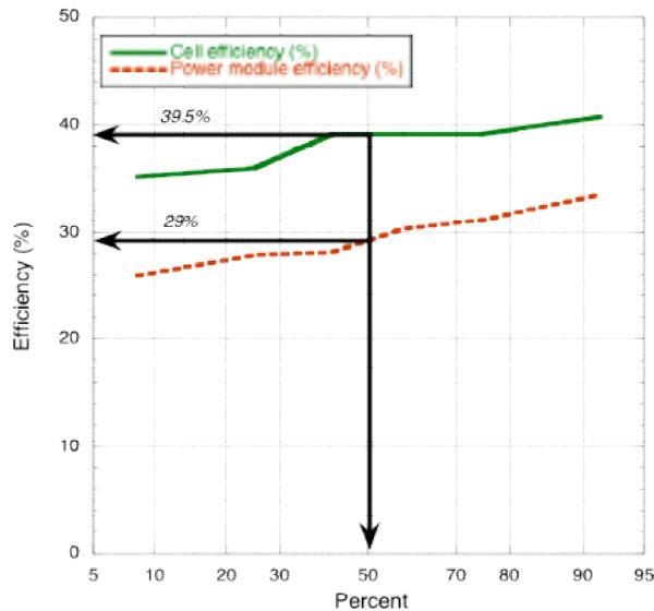
Figure 15 Measured efficiencies in the power module on stack- and system level.
