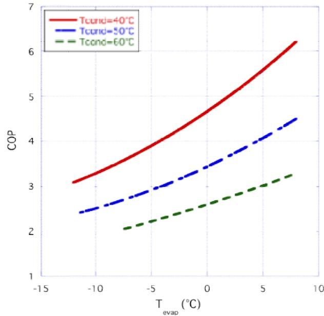
Figure 11 Typical temperature dependency of COP-values [ref]
