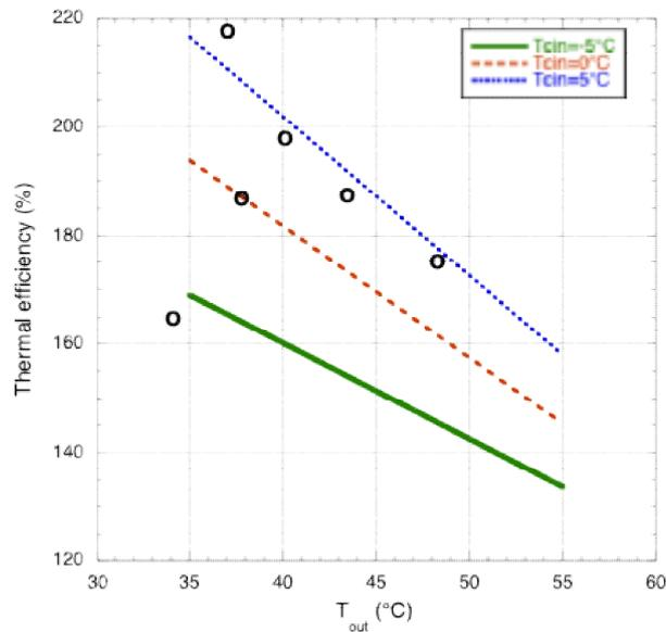
Figure 18 Thermal efficiency as a function of temperature levels for the evaluated system. Experimental points shown in the figure.
