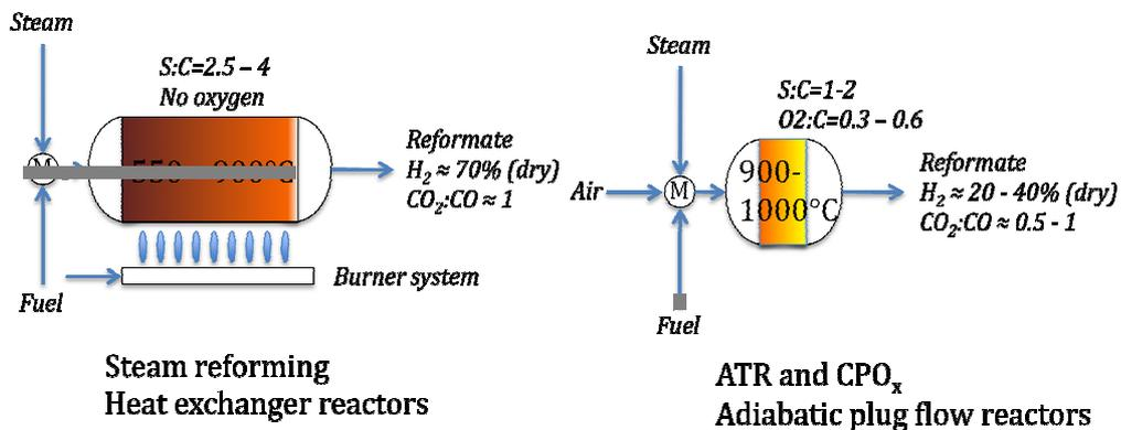
Figure 4 Various reformer technologies
