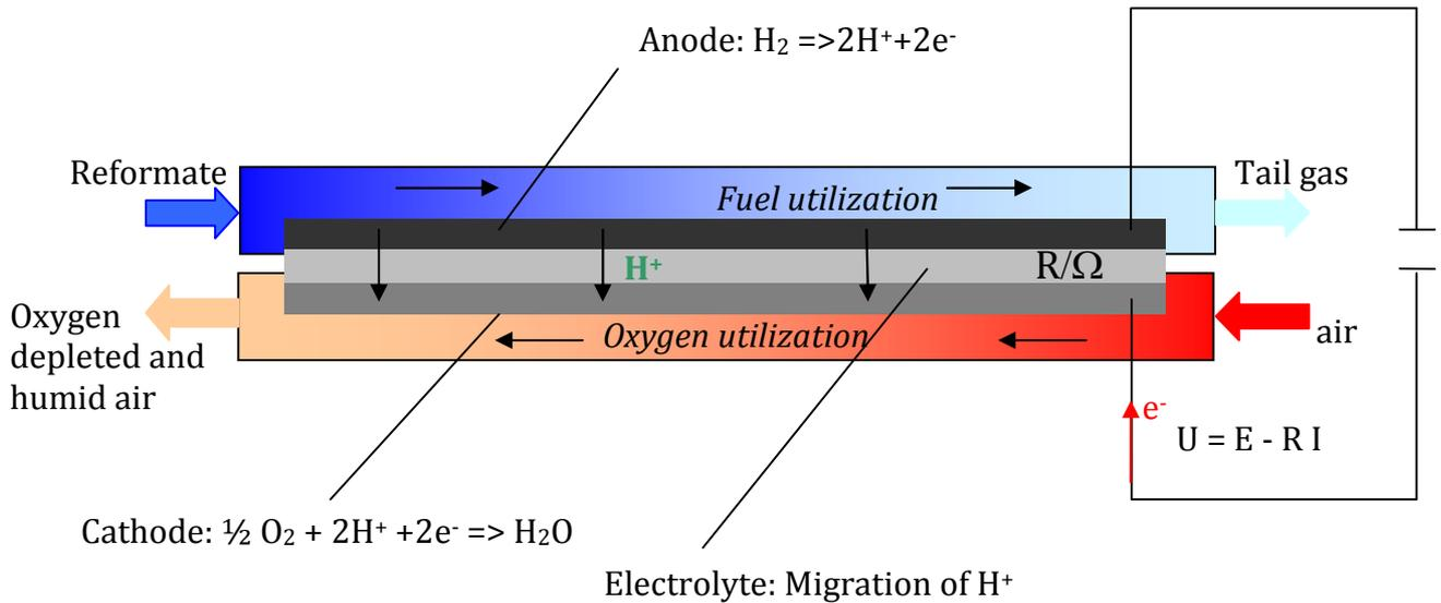
Figure 9b, Polymer Electrolyte Fuel Cell
