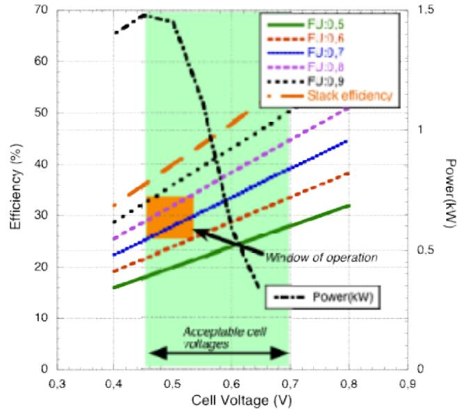
Figure 16 Efficiency of power module at different values of the cell voltage and fuel utilization. Power production versus cell voltage is given in the same diagram.
