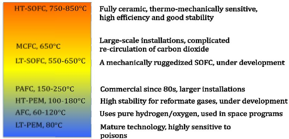
*Figure 5 Different fuel cell technologies*
