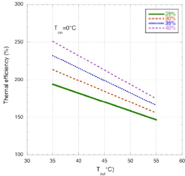
Figure 17 Thermal efficiency vs. the efficiency of the power module.  $T_{out}$  is the outlet temperature from the system.
