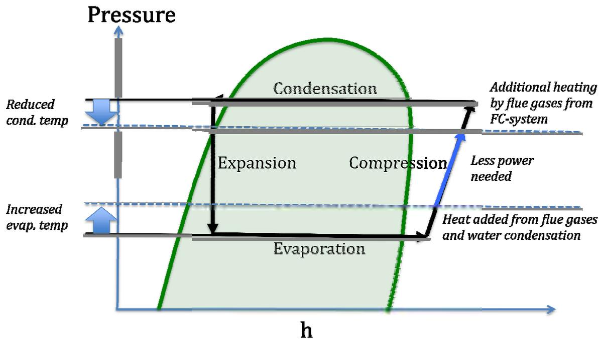
Figure 12 How we can shift COP to higher values
