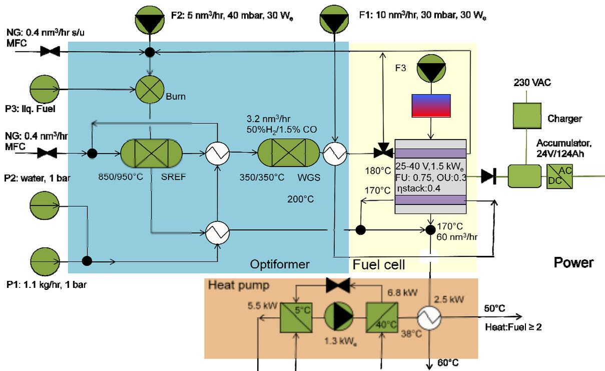
Figure 13 System lay-out and calculated data. Optiformer – proprietary reformer technology to Catator, HT-PEM delivered by Serenergy a/s, Heat pump supplied by Nibe. Heat exchangers supplied by AlfaLaval.
