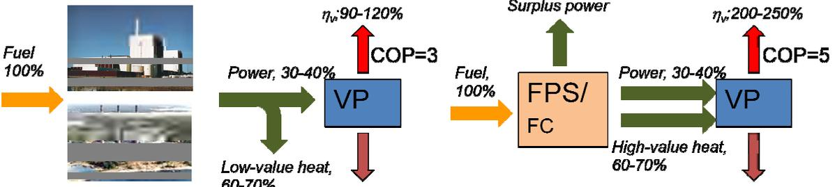
Figure 1 Thermodynamics of ComfortPower
