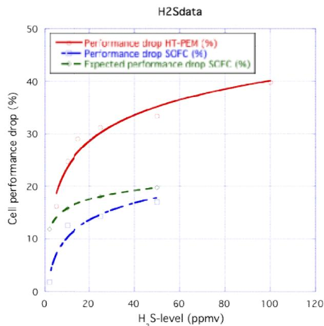
Figure 11 *S-sensitivity for HT-PEM- and SOFC cells. Tests performed at 170°C (HT-PEM) and 825°C (SOFC) with H<sub>2</sub>S-additiuon to a CPO gas containing ca 20% H<sub>2</sub>. Expected performance drop according to Hansen for the SOFC-cell [14] enclosed.*
