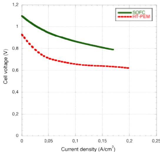
Figure 10 Fuel cell characteristics with reference gas ( $H_2/N_2$ -mixture) at 70% fuel utilization.
