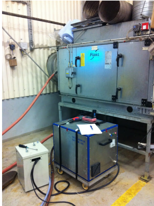
Figure 14. Photo of Deodoron when connected to the ventilation stream at Hall 2 for waste separation at Sobacken waste treatment plant.
