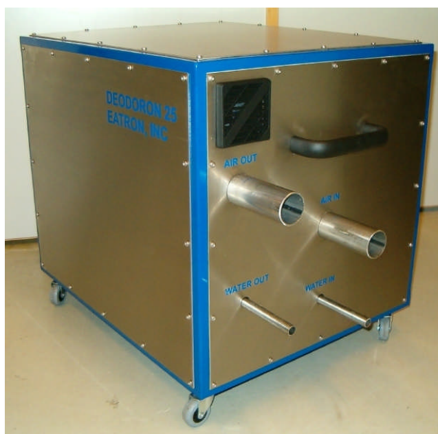
Figure 5. A photo of Deodoron – A catalytic, recuperative combustion unit for odour emission reduction. Capacity ~ 20 Nm 3 /h.
