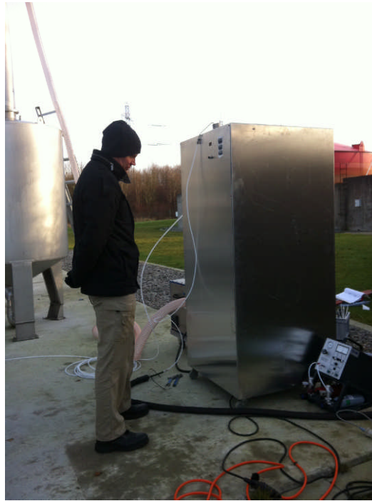
Figure 10. Photo of the MRO-unit connected to the rest gas out from the biogas upgrading plant at Källby, Lund.
