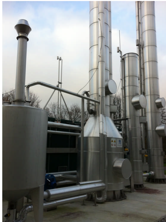
Figure 9. Photo of Malmberg's water scrubbing process positioned at Källby's waste water treatment plant, Lund. Design capacity= 200 \text{Nm}^3/\text{h} of raw biogas.
