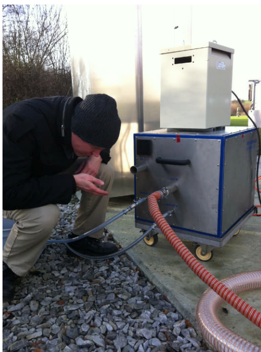
Figure 12. Smell tests of the purified air out from Deodoron when connected to the rest gas, up-stream the carbon cartridge, out from the biogas upgrading plant at Källby.
