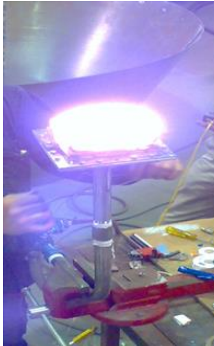
Figure 5. Burner at 1380°C with stable flameless combustion.
