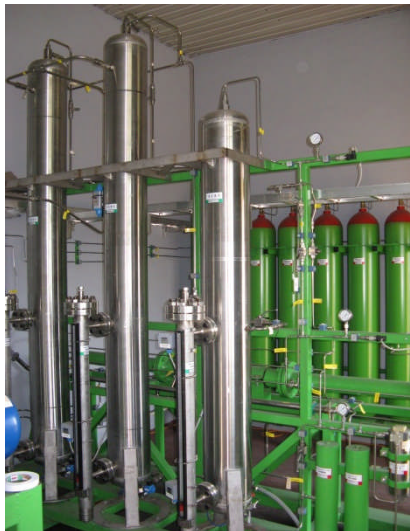
Figure 40 The columns performing the separation of carbon dioxide from the biogas in the Metener biogas upgrading system. Image from Metener Oy.
