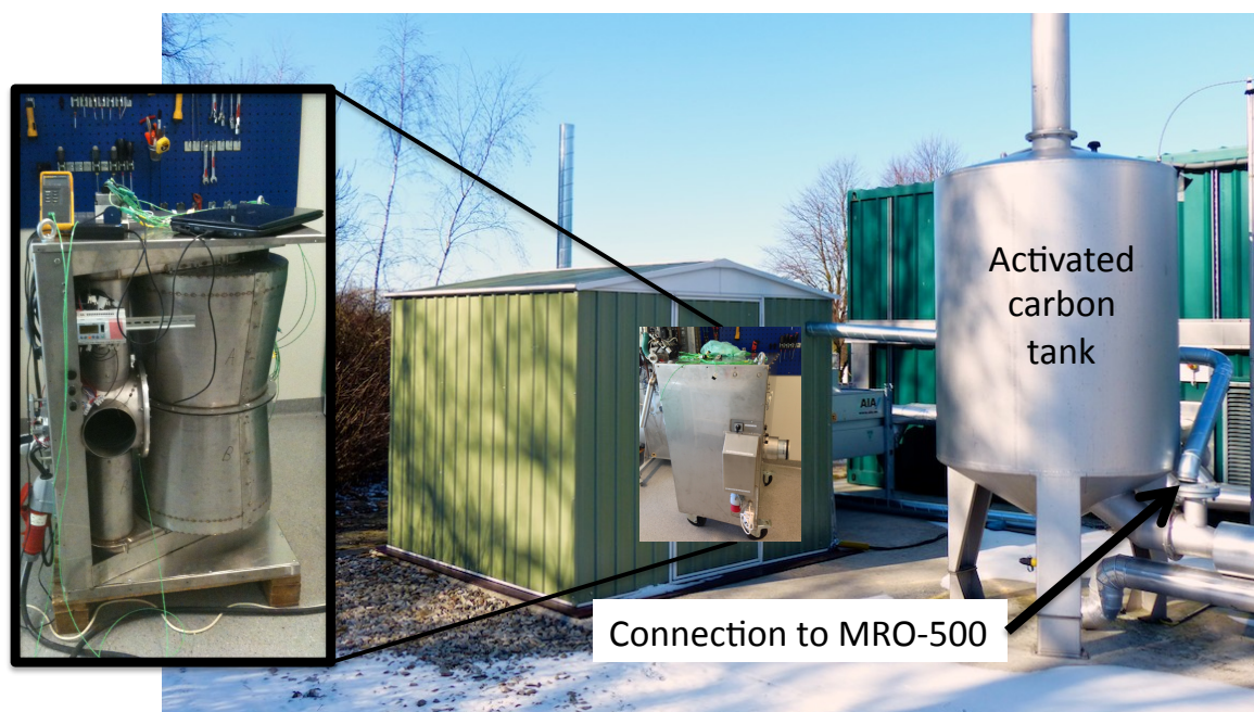
Figure 13. Installation of MRO-500 unit at Källby biogas upgrading plant. The unit is connected to the exhaust tube up-front the activated carbon tank.
