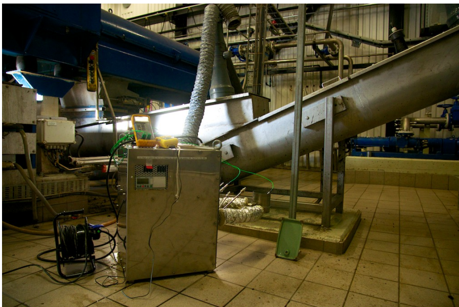
Figure 17. Evaluation of DEO-100 unit at dewatering press for sludge at NSVA municipal water treatment plant in Landskrona.
