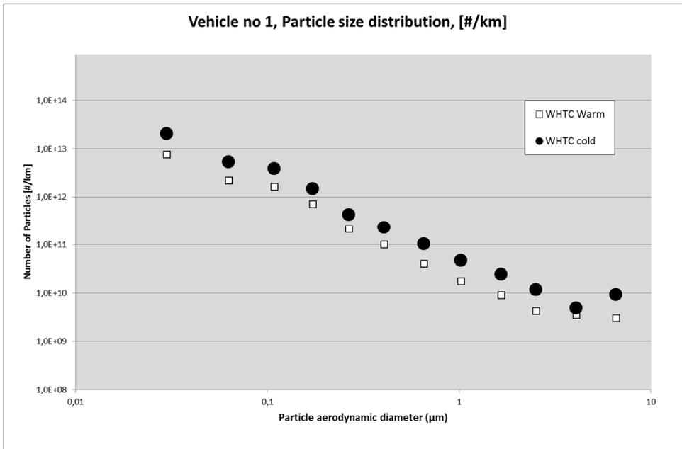
Figure 5. Particle size distribution of vehicle no 1, comparing the warm and the cold tests
