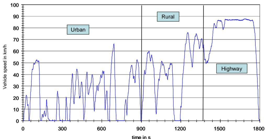
Figure 1. The WHVC/WHTC test cycle
