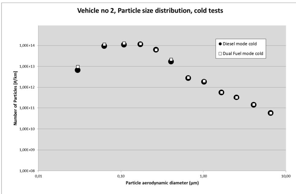
Figure 10. Particle size distribution of vehicle no 2, comparing cold tests when operating in DDF mode vs Diesel mode
