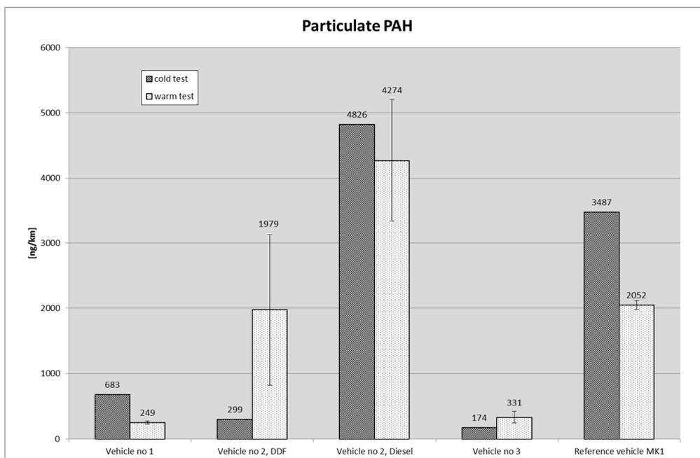
Figure 20. Particulate PAH, all vehicles, warm and cold tests
