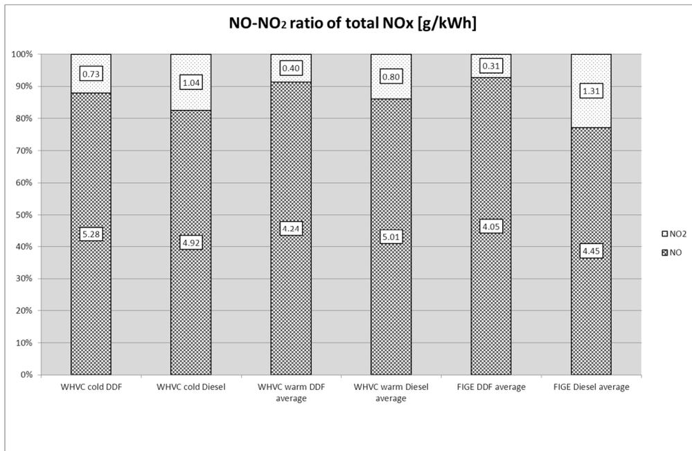
Figure 2. NO/NO<sub>2</sub> ratio of total NO<sub>x</sub> from vehicle no 2
