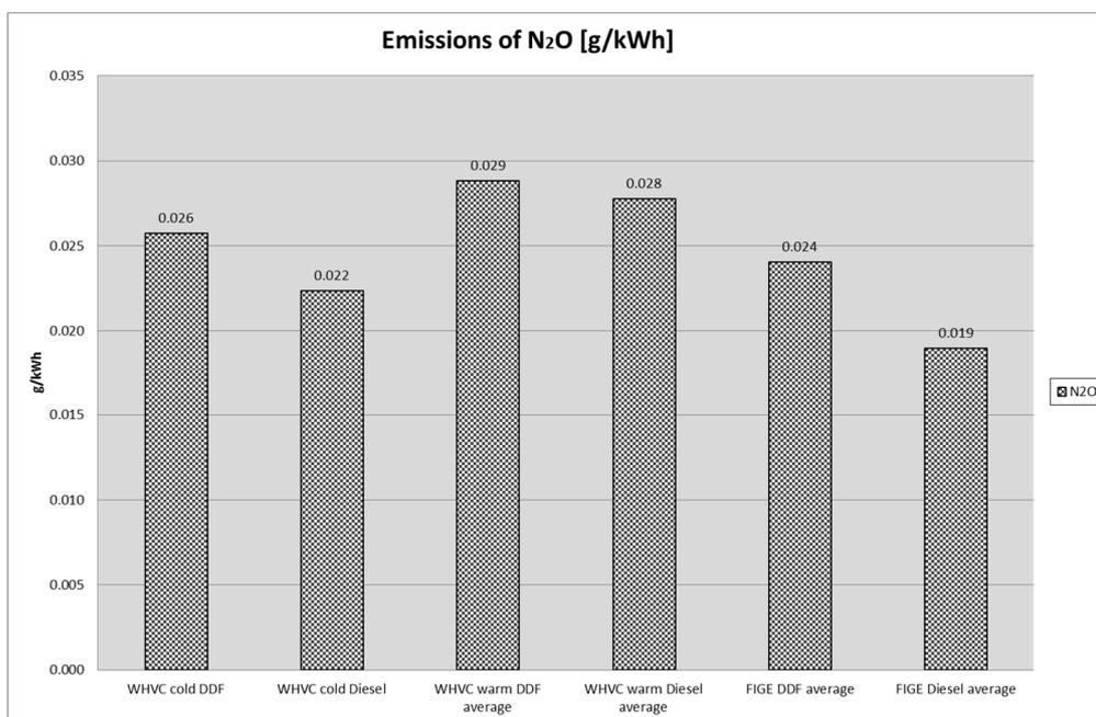
Figure 3. Emissions of N<sub>2</sub>O from vehicle no 2
