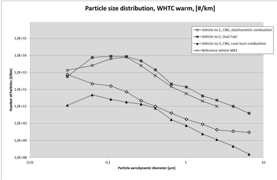
Figure 11. Particle size distribution of all tested vehicles during the warm tests
