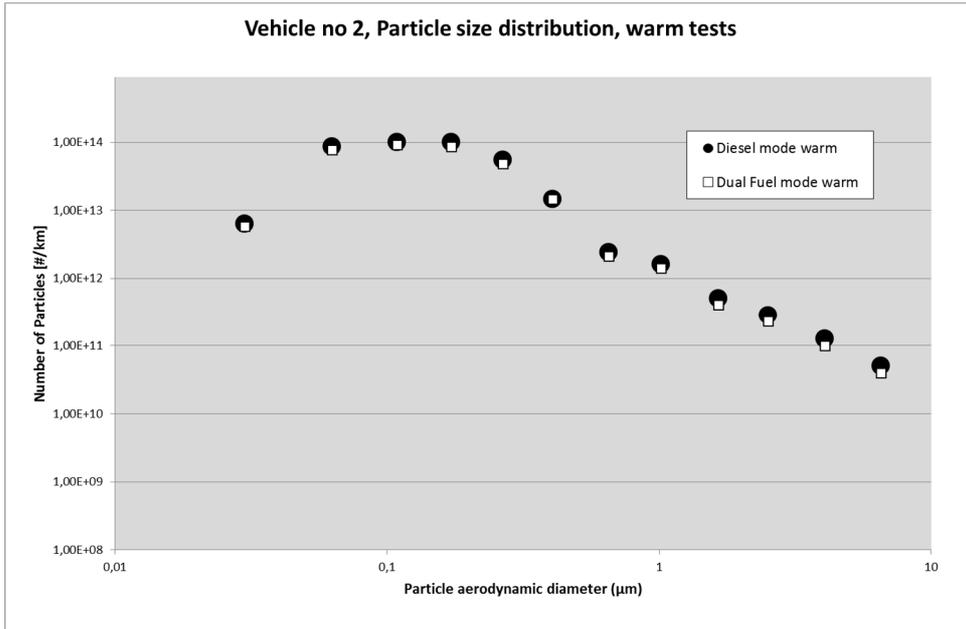
Figure 9. Particle size distribution of vehicle no 2, comparing warm tests when operating in DDF mode vs Diesel mode
