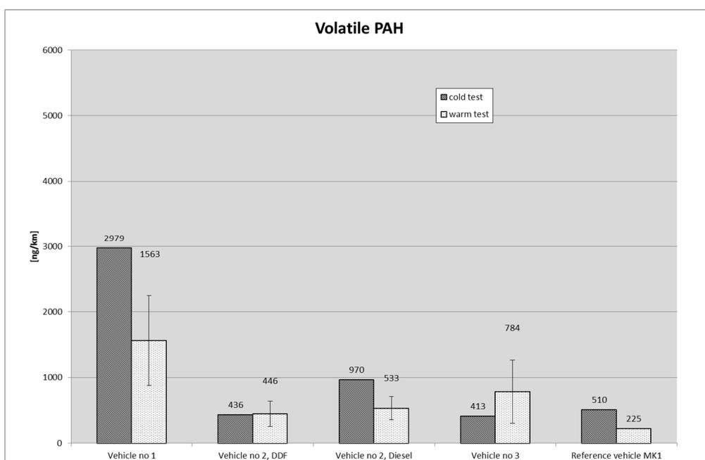
Figure 19. Volatile PAH, all vehicles, warm and cold tests
