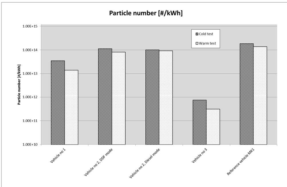
Figure 12. Particle number of all tested vehicles
