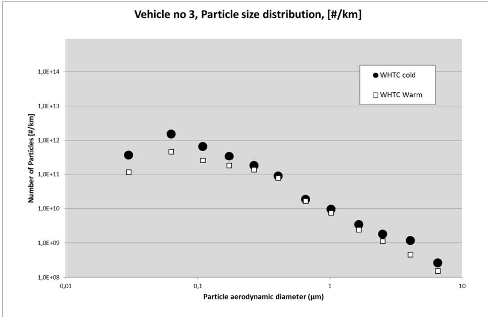
Figure 7. Particle size distribution of vehicle no 3, comparing the warm and the cold tests
