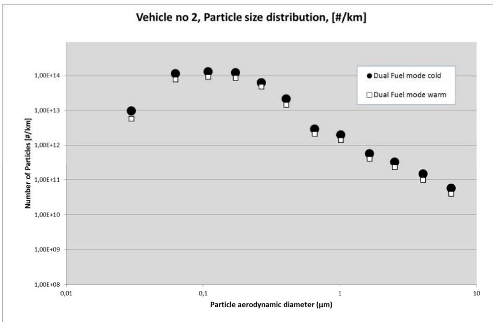
Figure 6. Particle size distribution of vehicle no 2, comparing the warm and the cold test when operating in DDF mode
