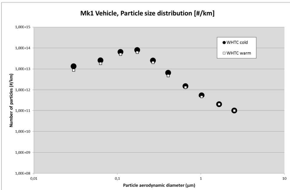
Figure 8. Particle size distribution of MK1 vehicle, comparing the warm and the cold tests
