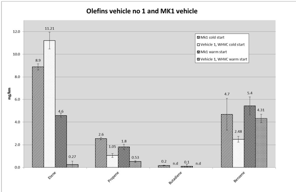
Figure 4. Olefins from vehicle no 1, cold start and warm start
