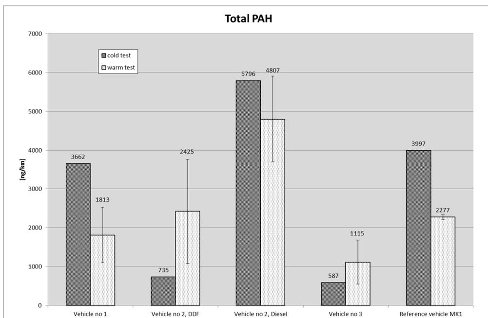
Figure 18. Total amount of PAH, all vehicles, warm and cold tests
