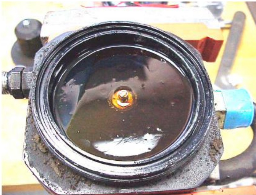
Figure 1.2: Example of oil deposition in the regulator [10]
