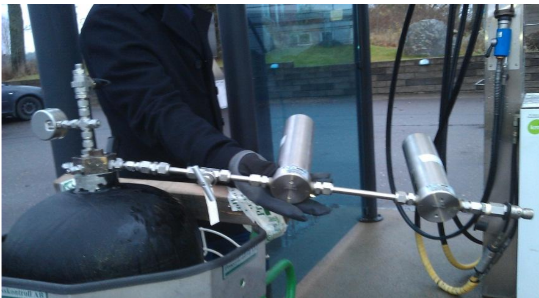
Figure 5.4: Third sample line with filter house and coalescing filters
