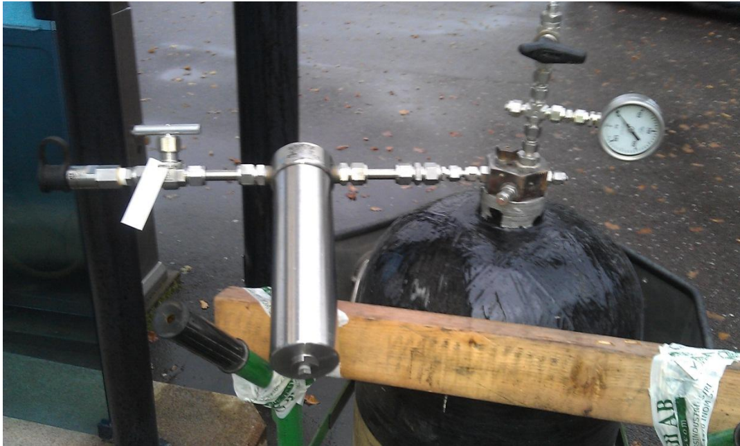
Figure 5.3: Second sample line with filter house and coalescing filters
