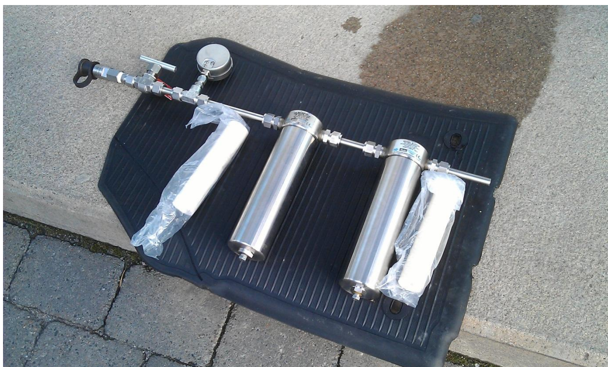
Figure 5.2: First sample line with filter house and coalescing filters
