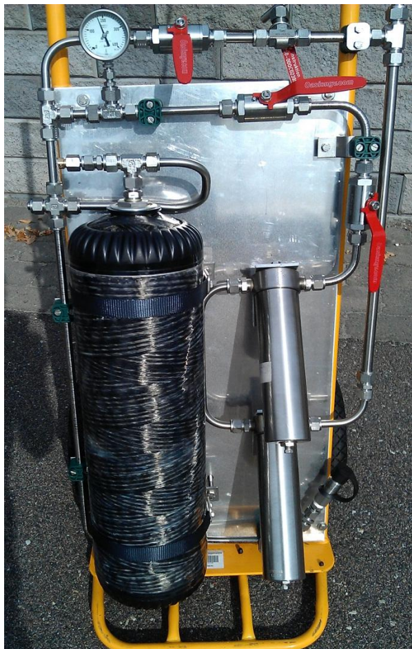
Figure 5.7: Picture of the sampler for oil determination at dispensers
