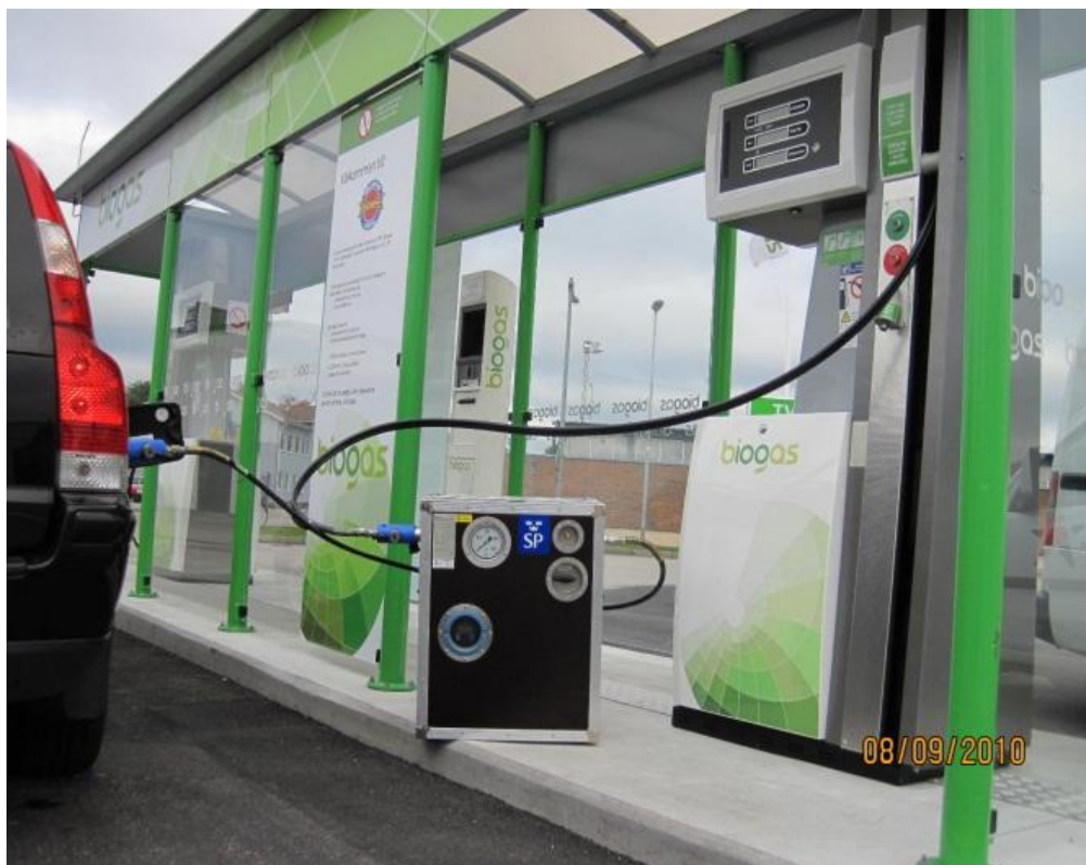
Figure 4.9: The flowmeter device connected to the pump and the vehicle
