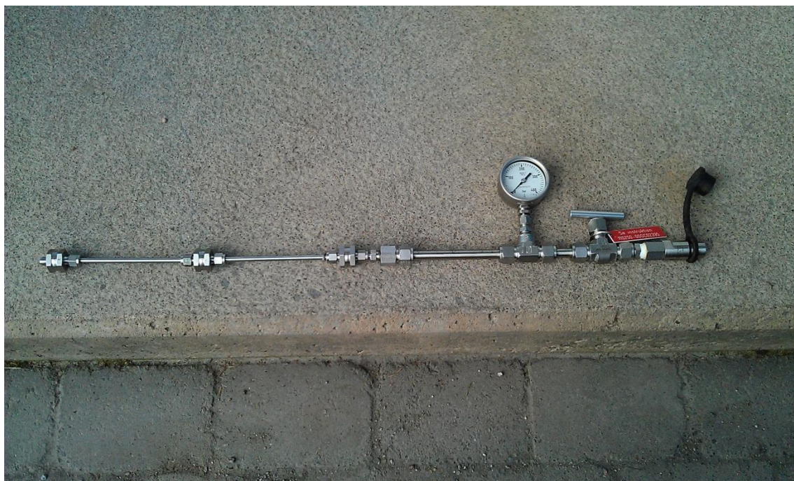
Figure 5.1: First sample line with tubes packed with adsorbent Chromosorb
