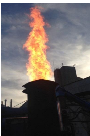
Figure 21. Combustion of syngas from gasification tests at the test plant.
