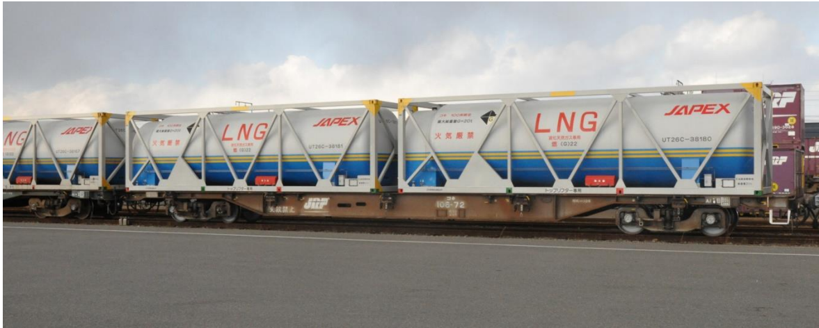
Figure 27. Loaded LNG containers on top of a railcar awaiting further transportation from Tomakomai to the destination Kushiro. Photo: Martin Ragnar.
