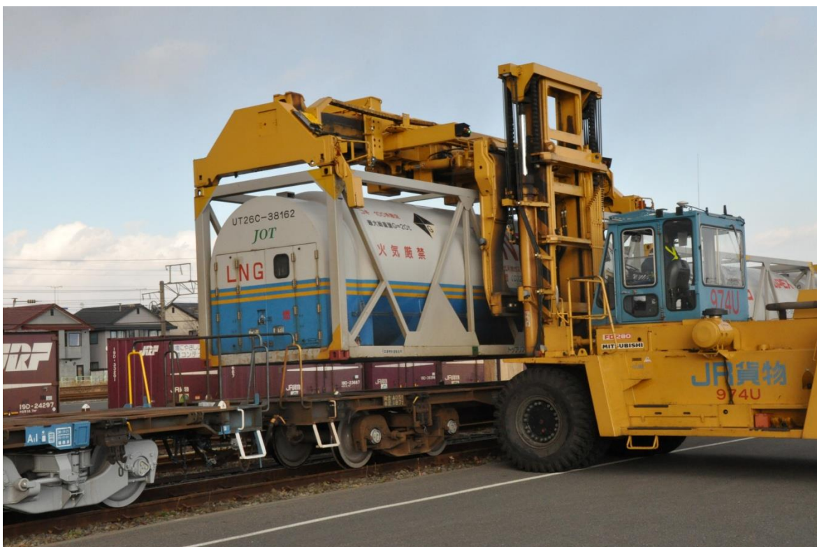
Figure 26. The loaded LNG container is fitted into its right position on the railcar by the top lifter. Photo: Martin Ragnar.
