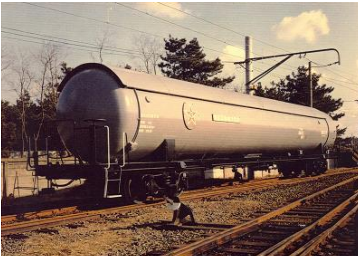
Figure 11. Specially designed LNG railcar for Tokyo gas, courtesy of JAPEX.
