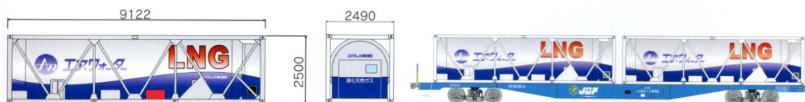
Figure 22. Air Water's LNG containers for trailers and railcars illustrated in a brochure by Air Water.
