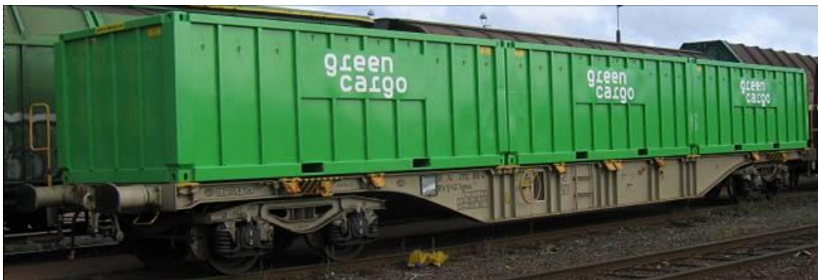
Figure 13. Green Cargo railcar type Sgnss here loaded with three 20 feet containers. This railcar could also handle two 30 feet LNG containers. Courtesy: Green Cargo.
