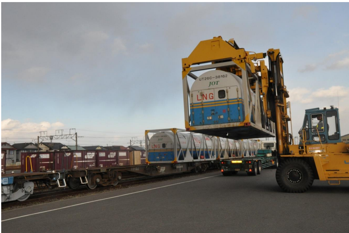
Figure 25. The loaded LNG container is lifted off from the trailer, which drives away. The top lifter holds the container in a steady grip and transfers it onto the waiting railcar. Photo: Martin Ragnar.
