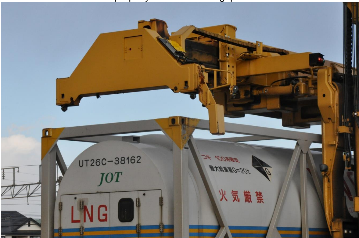
Figure 28. The top lifter has several security points to ensure the container is kept in a steady grip. When all points are correctly fitted a red light turns green and the driver could safely lift the container. Photo: Martin Ragnar.
