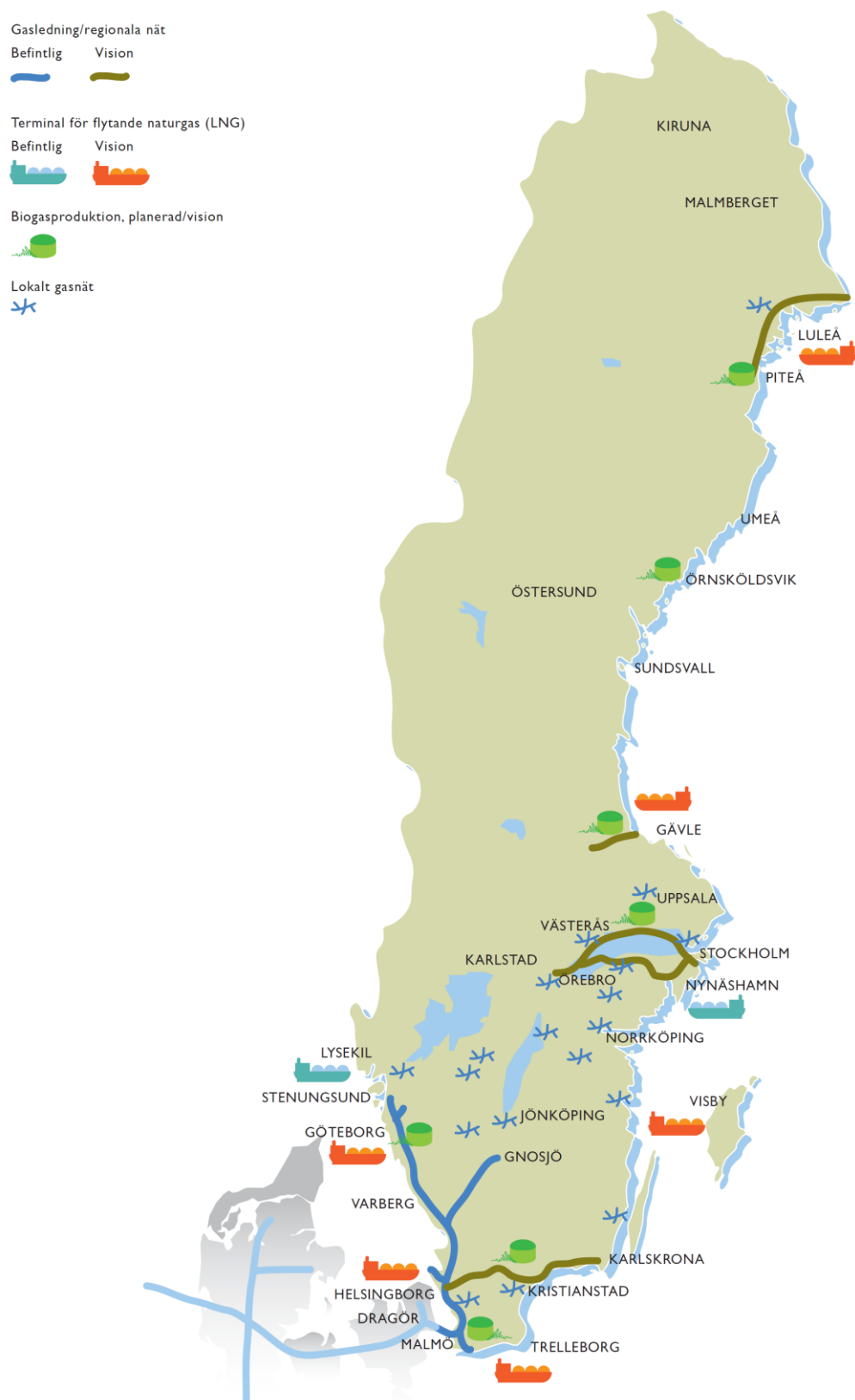
Figure 2. The Swedish gas grid. Malmberget, indicated on the map, is located very close to Gällivare, discussed in the text. Svappavaara, discussed in the text, is located some 100 km east of Kiruna. Source: Swedegas AB.
